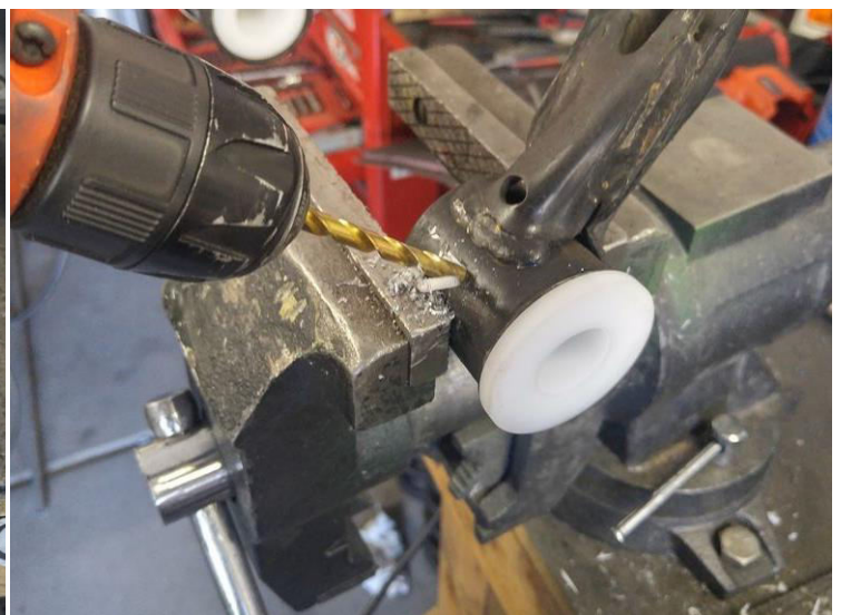
Fig. 9 drill through the control arm into the bushing bore
