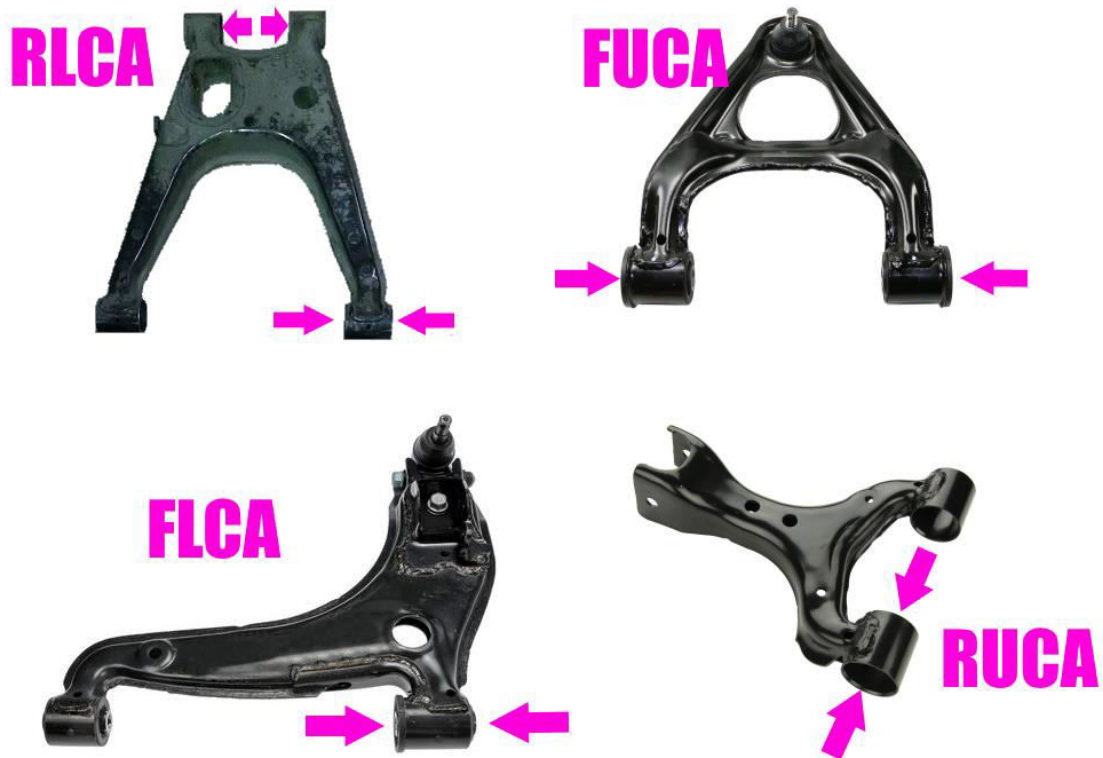
Fig. 7 Press bushings in according to the pink arrows.
