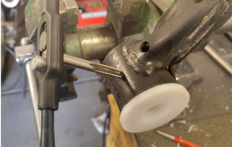
Fig. 10 Tapping to 1/4-28 for grease fittings.
