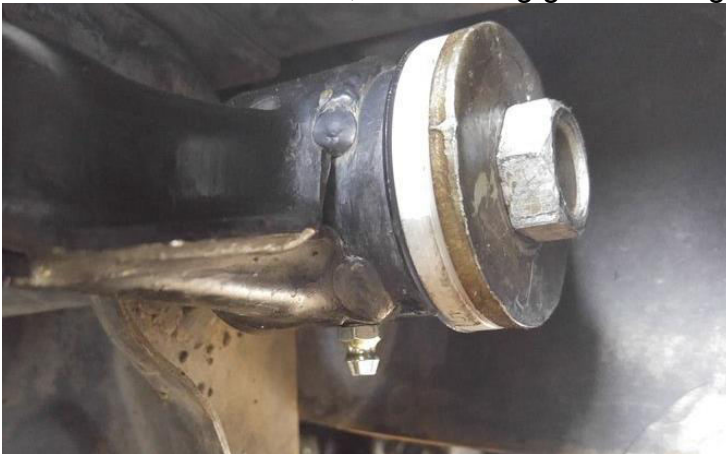
Fig. 11 FUCA- short fittings, installed straight down pointing at the ground
