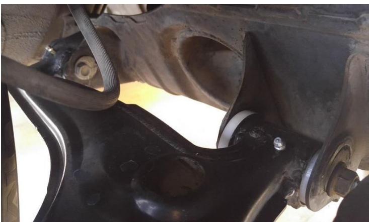
Fig. 12 LCA inners (all 8) - long fittings, installed in the "hole" of the bushing bore gusset. See Fig. 13 for clarification. Install the fittings into the poly locations (LCA inner rears) prior to installing poly in the next step. Deburr the ID as necessary for the poly locations, after drilling and tapping.
