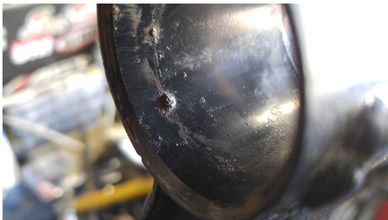
Fig. 6 Rust blob on the ID of a control arm bushing bore that needs to be wire brushed out.
