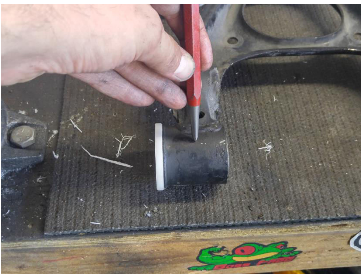
Fig. 8 marking the drill location with center punch
