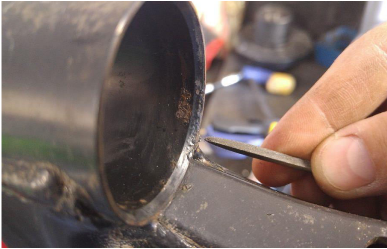
Fig. 5 Weld spatter from when the arms were originally manufactured that needs to be filed down so the bushing seats all the way.
