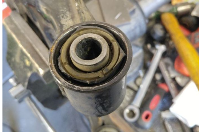
Fig. 4 Flange removed. (FUCA pictured)
