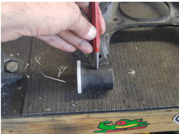
Fig. 5 Always center punch before drilling
