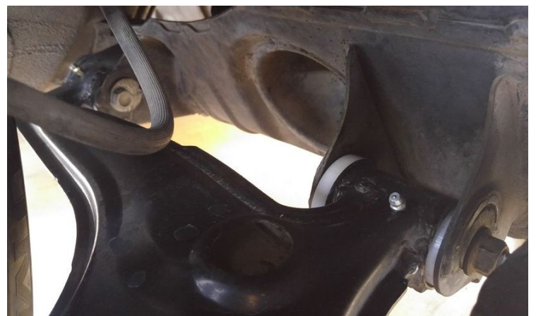
FLCA: long fittings, go in the hole in the bore gusset on the top side of the arm
