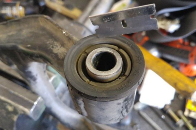
Fig. 3 Flange to be cut/torn off. (FUCA pictured)
