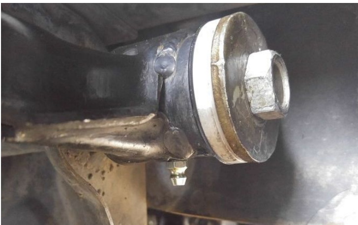
FUCA: short fittings, points at ground when installed
